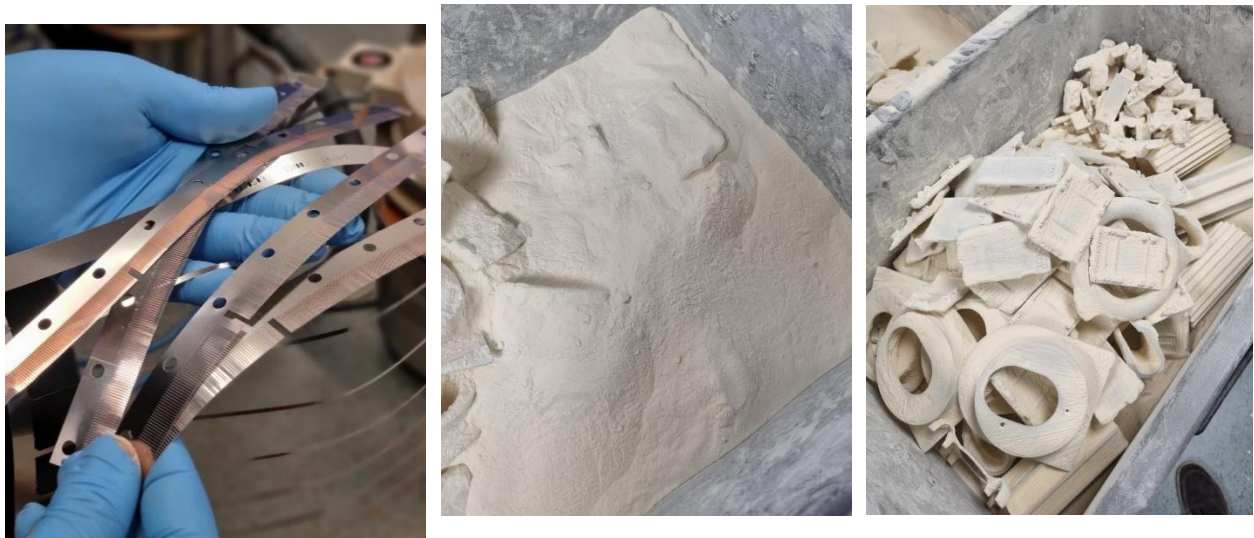
Figure 23 Residual printheads Resin waste: dust and failed parts.
