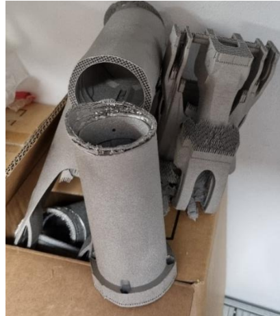
Figure 25: Titanium waste: supporting structures and failed parts.
