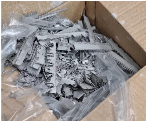
Figure 25: Titanium waste: supporting structures and failed parts.
