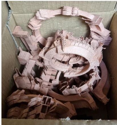
Figure 24: Copper waste: dust, failed parts and supporting structures.
